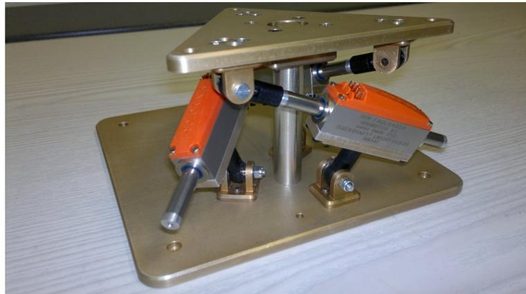
Figure 2.1: 3D rotary motion stabilizing platform designed in RoLab.
